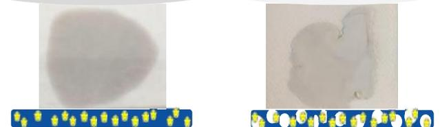
PVDF films were processed by Dr. blade casting with 30 μm thickness and 0.1 wt.% nanoparticle loading. Porous and non-porous substrates were generated by controlling the drying temperature to promote "temperature Induced phase separation (TIPS)" or to inhibit it.
