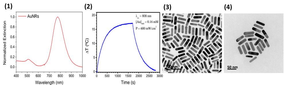
**Figure 2.** AuNRs were characterised using UV-Vis spectroscopy (1), thermal response (2) and TEM (3, 4). Thanks to the LSPR situated at 780nm, AuNRs produced heat upon irradiation with an 808 nm laser. When irradiated with a power density of 660 mW/cm<sup>2</sup>, an increase in temperature of 17°C was recorded.
