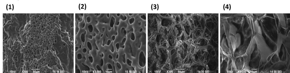
**Figure 3.** Structural characterization by SEM imaging of 3D-printed NIPAm-PEGDA based stimuli-responsive film after removal of the sacrificial material (1,2) and the cell containing layer composed of 5% GelMA – 1% alginate gel (3,4). Uniform porosity is observed.
