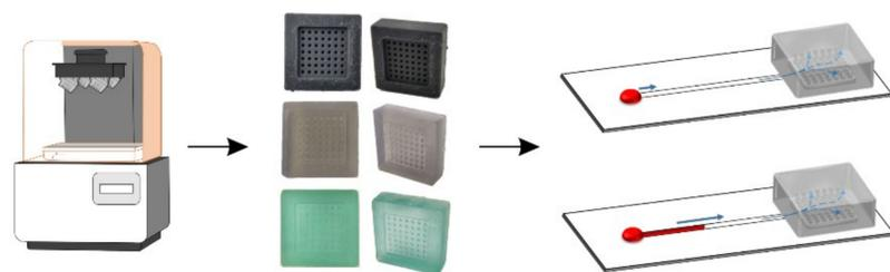
Scheme of the 3Dp-μPumps fabrication (SLA and DLP) and actuation principle.
