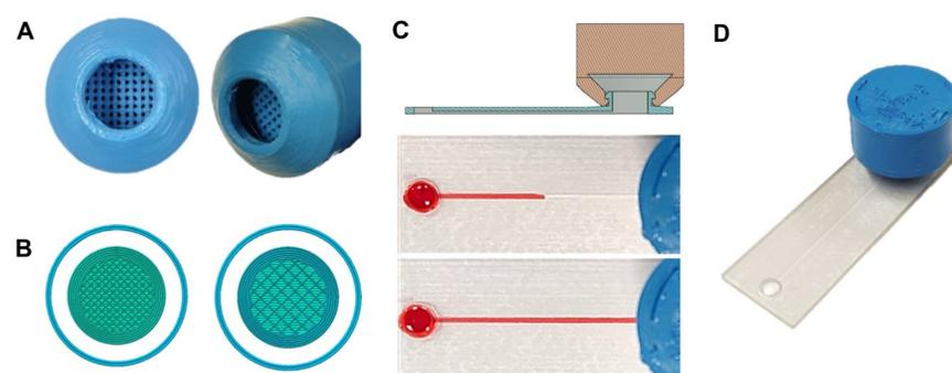
FDM 3Dp-μPumps manufactured with a different internal infill were connected directly to a 3D printed device without the use of a PSA layer.
