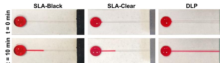
Pictures of a multilayer PMMA thermolaminated device connected to a SLA-black, SLA-clear and DLP 3Dp-μPumps at 10 min after loading the sample.
