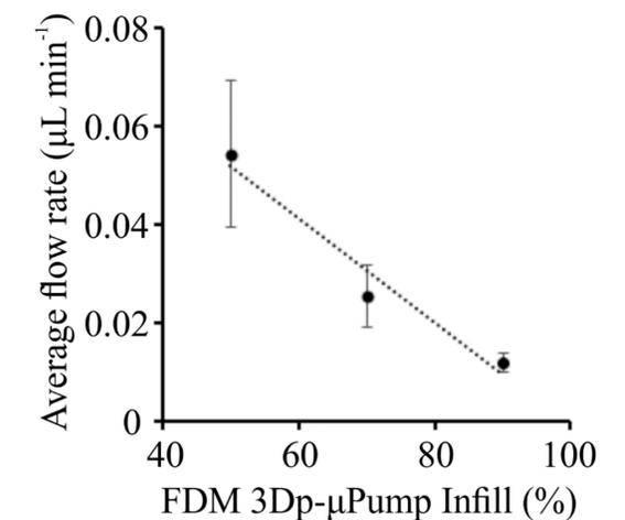
FDM 3Dp-μPumps flow rates characterization using increasing percentage of internal infill.
