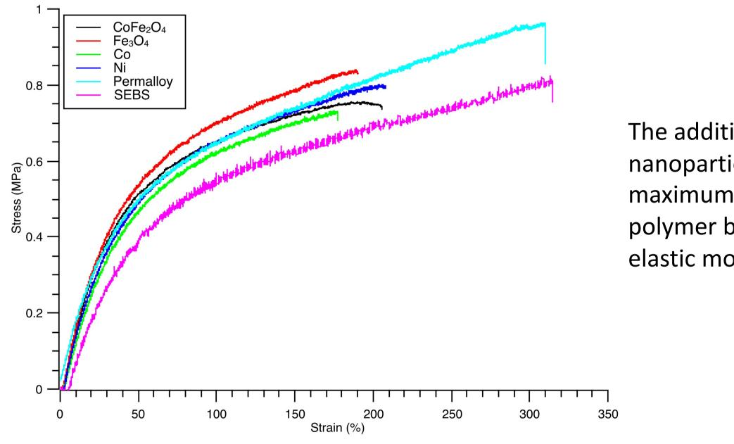
The addition of the magnetic nanoparticles decreases the maximum elongation of the polymer but also enhances the elastic modulus.
